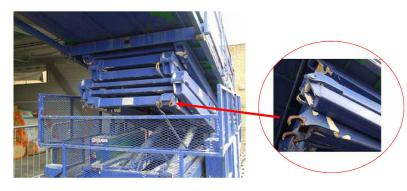
Initial examination identified oxidization, a suggestion of developing fatigue and fatal stress fractures. This quipment has been recovered for detailed examination by Skyjack and the HSE.
