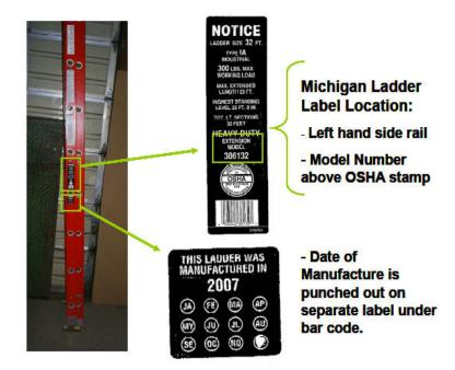
Ladders manufactured during September 2007 and October 2007 but with two green dots near the bottom of the left side base rail have already been inspected or repaired and are not affected.
